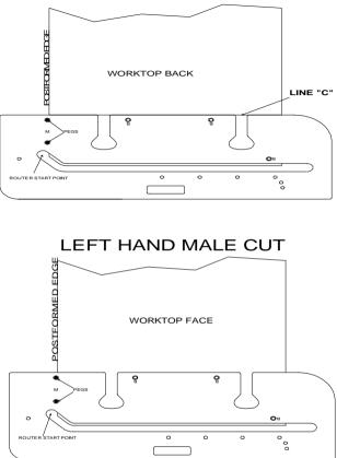
Set the jig onto the worktop as shown and clamp firmly in place. Again, always starting the router from the extreme left of the slot, use the side of the slot nearest to you setting the plunge depth to no more than 10mm per pass, remove the waste.
