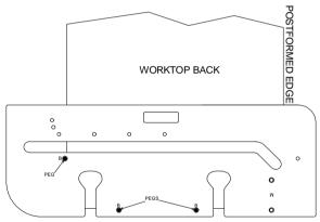
Again with the worktop face down set the jig in place (jig face up for right hand male bolt slots and jig face down for left hand male bolt slots). Clamp the jig in place as before and repeat the routing procedure described on the previous page.
