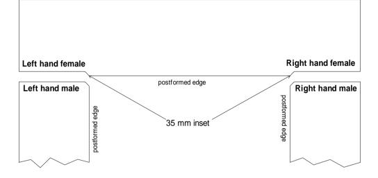
The construction shown above is the easiest to fit and should be used if possible. Another layout is shown below but this requires careful measurement and recovery from error measurement and cutting "worktop 3" is limited.
