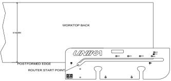
Fig. 1 shows the female mitre set-up for a 616mm wide worktop, for other work top widths the peg used to set the cut length should be changed.
