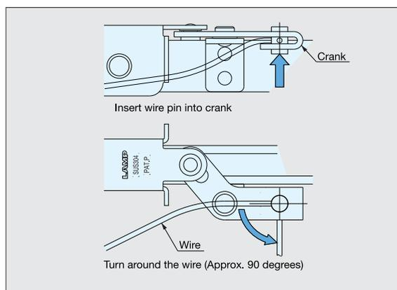
Installation of lock-release wire (WR and WL type only)
