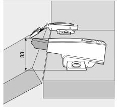
For all hinges with a straight hinge and a 3 mm spaced mounting plate. Use also for 95° profile door hinge with 0mm spaced plate.
