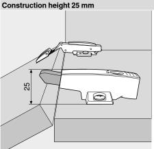
For all hinges with a straight hinge arm and a 0 mm raised mounting plate. Exception: 95° profile door hinge
