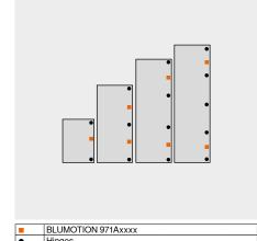
For optimal BLUMOTION effect, BLUMOTION 971A should be attached to the centre between the hinges. For high and heavy doors, we recommend using an additional BLUMOTION 971A between an additional hinge pair.
