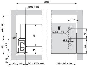
\* Recommendation/Minimum dimension: 49.5 mm/Tipmatic Soft-close: 58 mm
