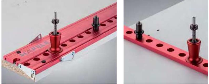
The drilling jig is moved and fixed with the locating pin for longer rows of series drilled holes.
